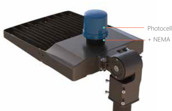
NEMA+Photocell 3-PIN: Lighting Switch 5-PIN: Expandable DALI or 0-10V Dimming 7-PIN: Expandable DALI and 0-10V Dimming
